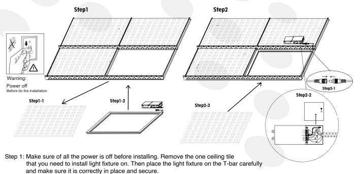
Step 2: Place the driver on top of the next ceiling tile. Connect the cable between the driver and the lighting fixture.
